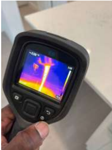
110 degrees at kitchen faucet
