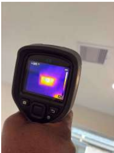
105 degrees heat output measured from hallway register
